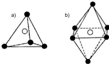
Figure 3 - (a) silicon tetrahedral structure e (b) aluminum octahedral structure.
