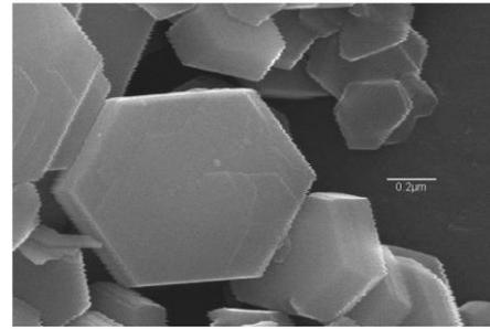
Figure 5 - the clays kaolinite crystals.
