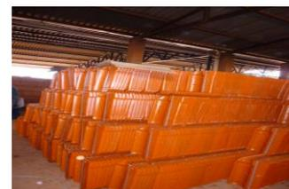
Figure 2 - Resinous tiles produced from the clay
